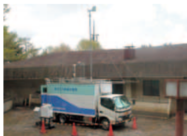
PM 2.5 research and measurement by air quality measurement vehicles
