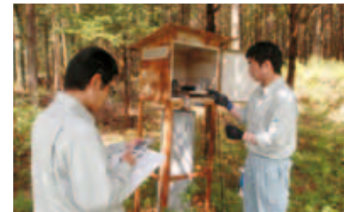
Measurement of groundwater temperature in observation well
